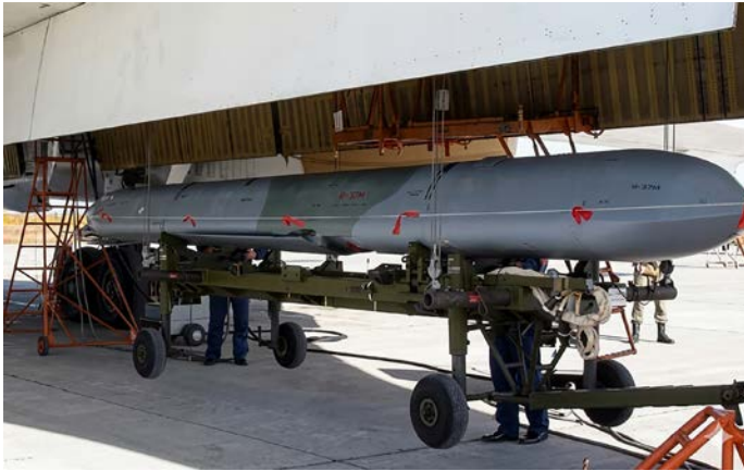
Figure 15 : Kh-101 cruise missile loaded in the weapons bay of a Tu-160 © Ministère de défense russe
