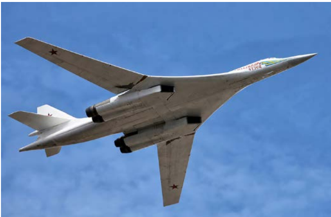
Figure 12 The Tu-160 with wings at maximum 65 degrees. Ultra-long subsonic range of action of the Tu-160M2 at low altitude with 2 x 6 fully internal Kh-101 cruise missiles in the weapons' bay is 1,740 NM / 3,230 km). © Vitaly V. Kuzmin, CC BY-SA 4.0
