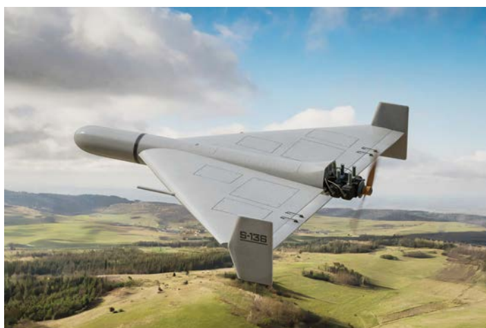
Figure 1 : Shahed 136: wingspan 2.5 m; length 3.5 m; weight 180 kg; explosive charge 40 kg; range 1,700 km ; price $20,000. © Adobe stock
