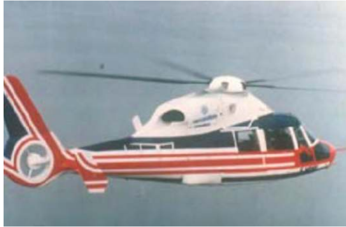
Figure 189 - DGV 200 – 1989 – C_x S = 0,85 \text{ m}^2
