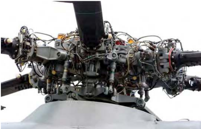
Figure 51 - Le moyeu repliable du SA 321 G © Photo DR/Airbus Helicopter
