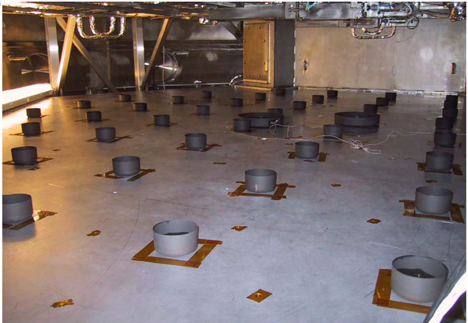
52 liquid mirrors are aligned on optical bench inside the chamber
