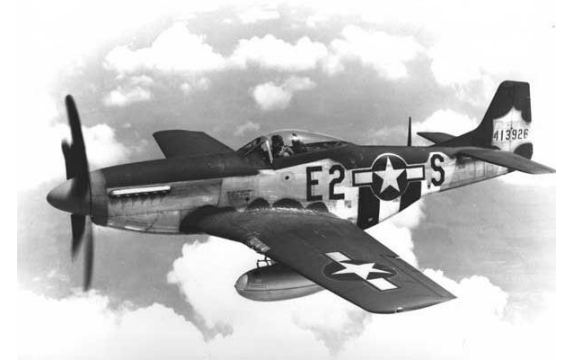
North American P-51 Mustang (1941). A laminar air foil was used at the design of the wings...
