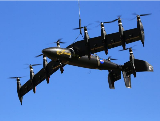
NASA 10-engine electric plane scaled test plane
