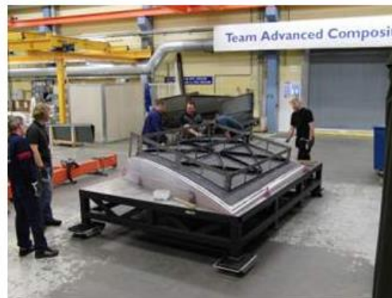
Current manufacturing of the Smart Wing integrated upper panel (SAAB)
